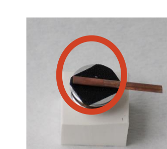
Copper electrode. The copper deposit is circled in red.
